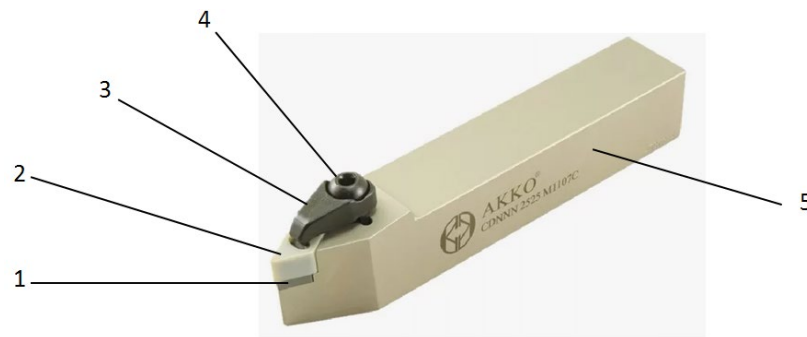
Figure 1. Ceramic cutting tool. 1-carbide backing plate; 2-mineral ceramic insert; 3- insert fastening; 4- differential screw; 5-tool holder.
