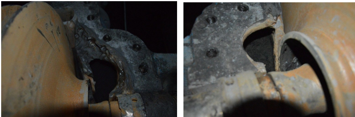
Figure 1. Severe abrasive wear, micro-trough, and local cavitation wear in the metal working parts of the slurry pump observed in industrial operation [4, 5, 13, 14].
